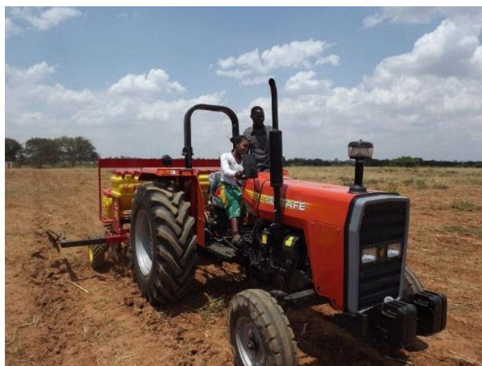
Figure 3. Training in field operation of a tractor-mounted no-till planter.
