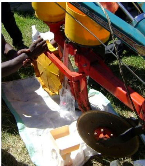
Figure 2. Calibration of a single-row no-till planter. The drive wheel is turned by hand and the seeds collected in a plastic bag attached to the seed outlet. Seeds can be counted and/or weighed to calculate seeding rates per ha.
